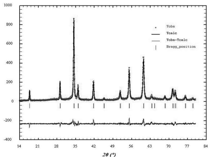
Fig. 2: XRD pattern of  $Zn_2SnO_4$ , sintered at 825 °C for 1 h.
