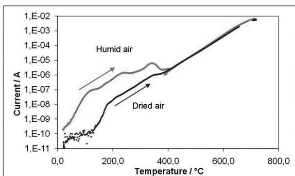
Fig. 5: Current vs temperature plot between humid and dried air
