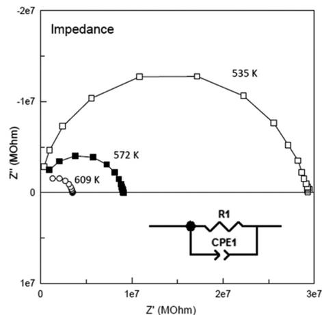
Fig. 9: Impedance plot for  $\text{Zn}_2\text{SnO}_4$
