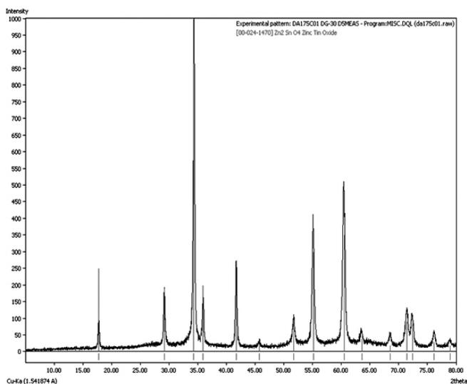
Fig. 1: XRD pattern of  $Zn_2SnO_4$  compared with database.
