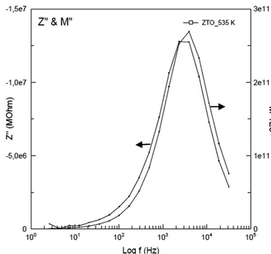
Fig. 10:  $M''$  and  $Z''$  spectroscopic plots for  $Zn_2SnO_4$
