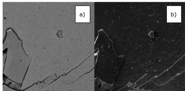
Fig. 4: a)  $Zn_2SnO_4$  backscattered electron image. b) Secondary electrons image for the microstructure of  $Zn_2SnO_4$  pebble, sintered at 825 °C for 1 h.
