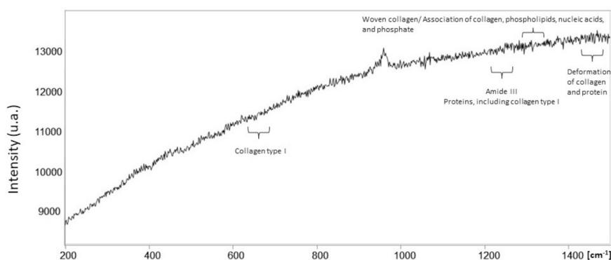
Fig. 2. Spectrum model and definition of analyzed bands.
