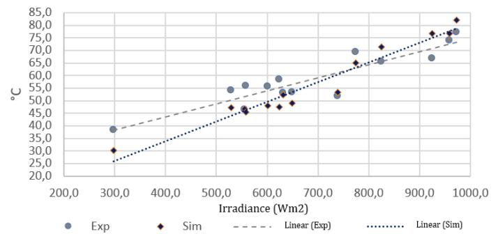
Figure 4. Aluminum plate temperature. Preparation by the authors.
