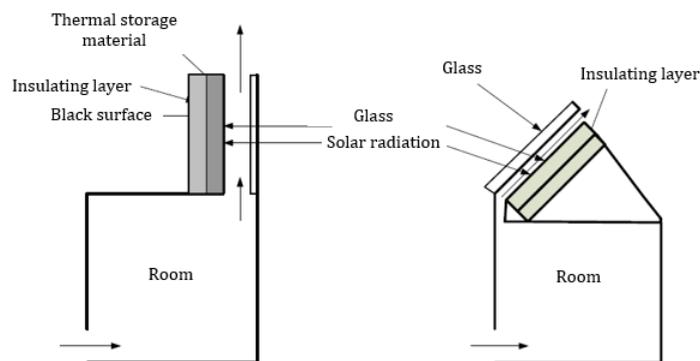
Figure 1. Solar chimney setups. Source: Harris & Helwig (2007, p. 136).
