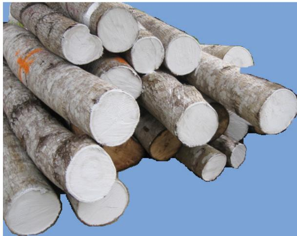
**Figure 2.** The logs of 7 yr-old *N. cadamba* cut into the billets.
