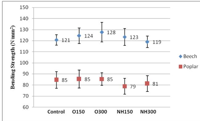
**Figure 2.** Bending strength (MOR) of the test panels.
