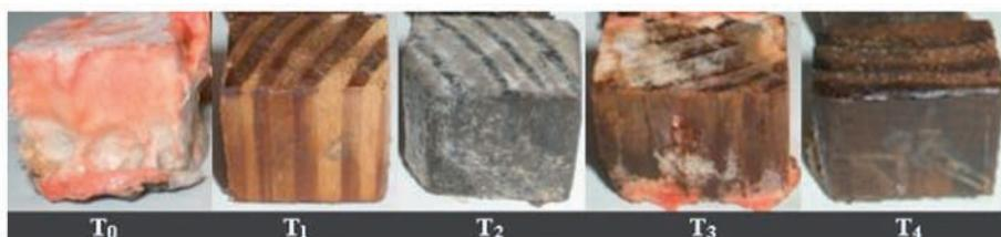
**Figure 5.** View on the test tubes after 3 months of culture with *Pycnoporus sanguineus*. Abundant colonization in the pinewood without impregnation (T<sub>0</sub>).
